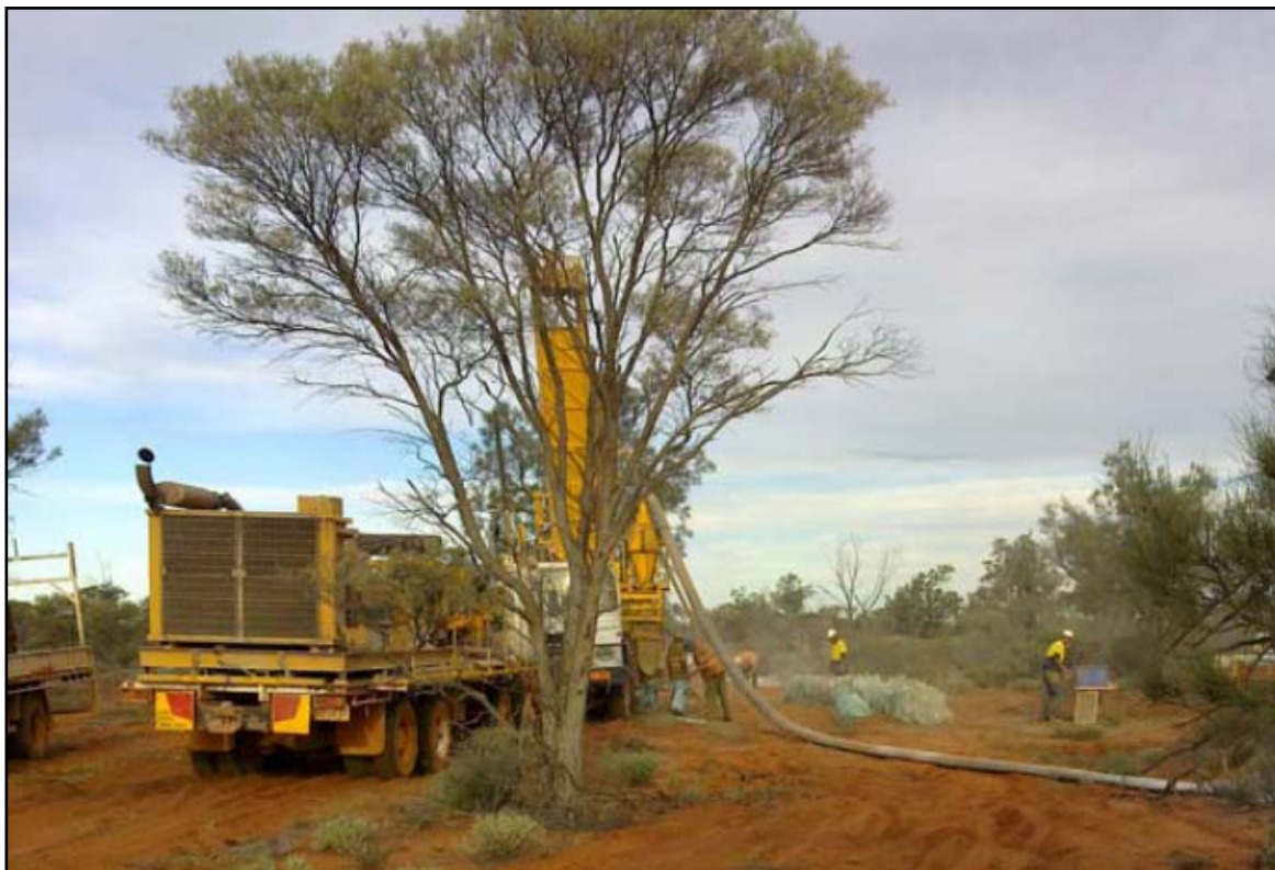
Figure 2 – RC drill rig at George Hill South 2, Gawler Iron Project.
