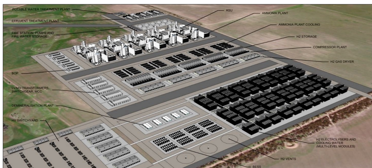
Figure 1: Key plant building blocks, Cape Hardy 5GW Advanced Fuels project (courtesy of Amp Energy).
