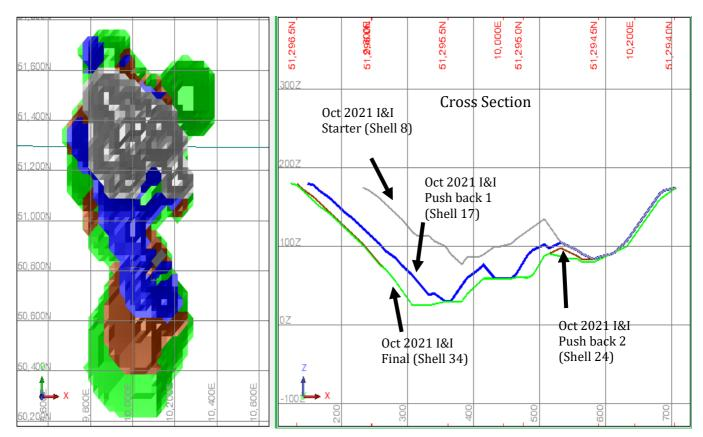
Figure 10 - Pit optimisation results for Indicated and Inferred Resource Estimate. Including Intermediate stages - Shell 8, Shell 17, Shell 24, Shell 34. Optimisation completed for silver price of \$A34.30/oz Ag.
