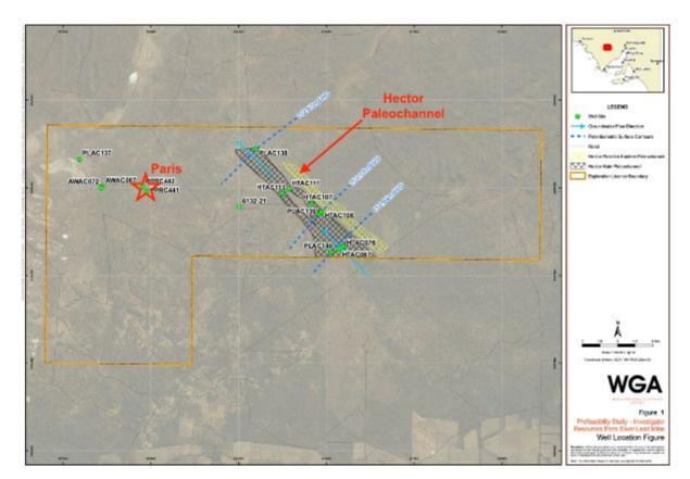
gravity, electromagnetic profiles and magnetic data indicated that the paleochannel footprint was likely sufficient to be considered as a water source for the deposit.
