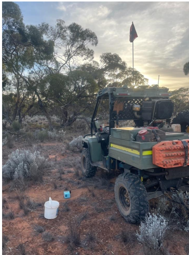
Figure 3: Tromino seismic sensor being positioned at Hector.
