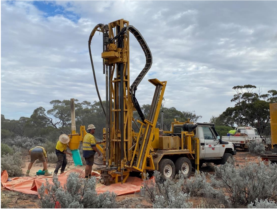
Figure 4: Aircore rig drilling a sterilisation hole at the planned Paris processing plant site.
