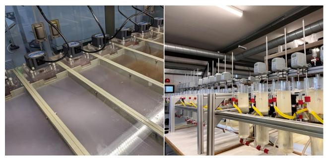
Figure 3: Ionic Technologies' demonstration scale solvent extraction (SX) circuit (left), and Ionic Technologies' Heavy REE SX circuit (right).
