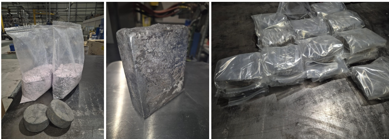
Figure 1: Neodymium ingots, after reduction, and Dysprosium (centre) and Terbium ingots (right) after Vacuum remelting (used with permission from LCM).
