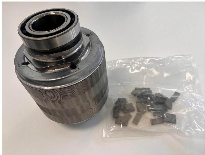
Figure 2: Left, representatives from Ionic Technologies meet Dennis Witt, Ford Innovation Manager (third from left) and Aaron Riley, General Manager LCM (far right) at Ford's Halewood e-motor manufacturing plant, UK, and right, e-rotor made using magnets produced via the supply chain, with spare magnets.
