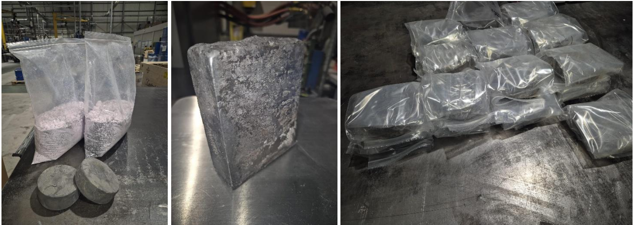
Figure 1: Neodymium ingots after reduction; Dysprosium (centre) and Terbium ingots (right) after Vacuum remelting (used with permission from LCM).
