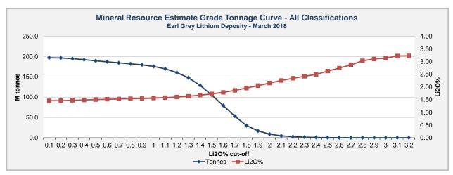
Figure 3: Grade tonnage curve for Earl Grey Mineral Resource Estimate - March 2018
