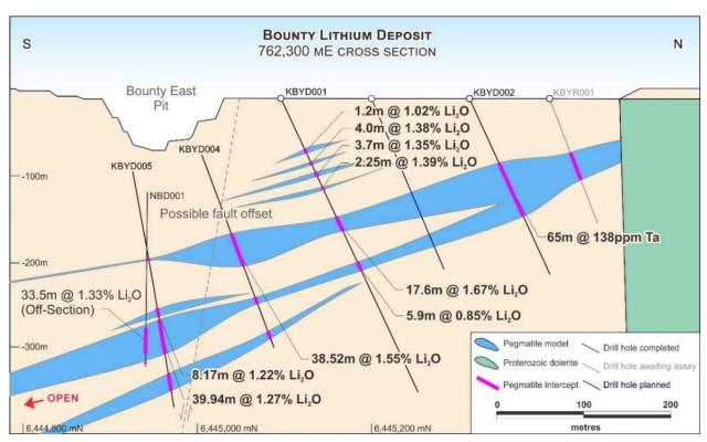
Figure 6: 762,300mE Cross section, Bounty mineralised pegmatite.
