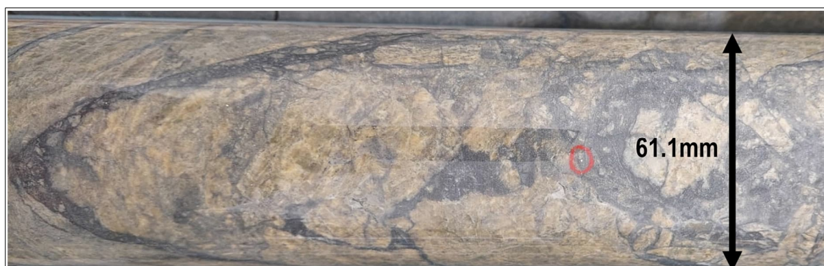
Photo 3. Visible gold zone (circled red) in hole 25ENDD002 at 293.3m down hole in dark sulphidic quartz veins within granite host rock. Drill core diameter is 61.1mm.
