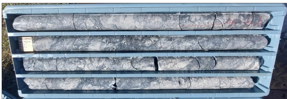
Photo 4. Dark sulphidic quartz veins and breccia within granite host rock in hole 25ENDD002 from ~332m-336m. Drill core diameter is 61.1mm.
