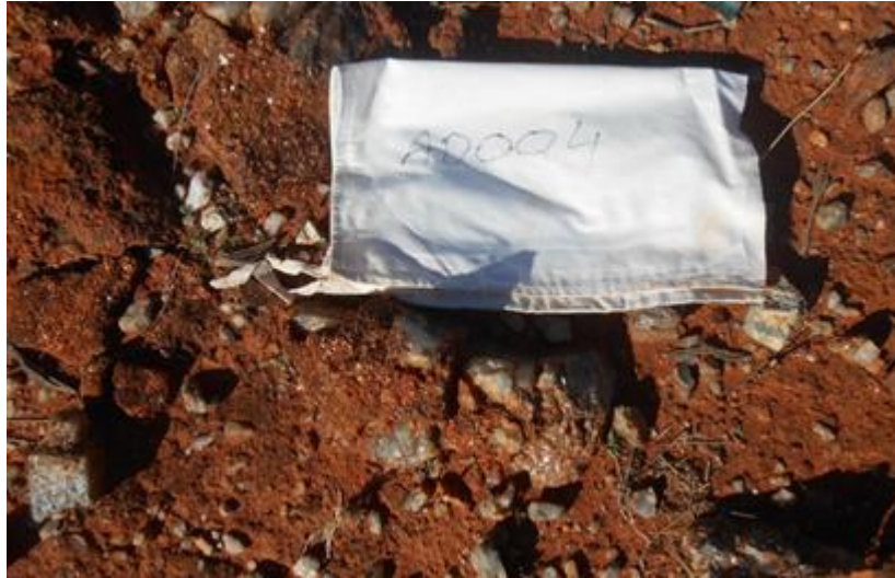
Figure 2: Pegmatite sample AD004, returning >5000ppm Rb.
