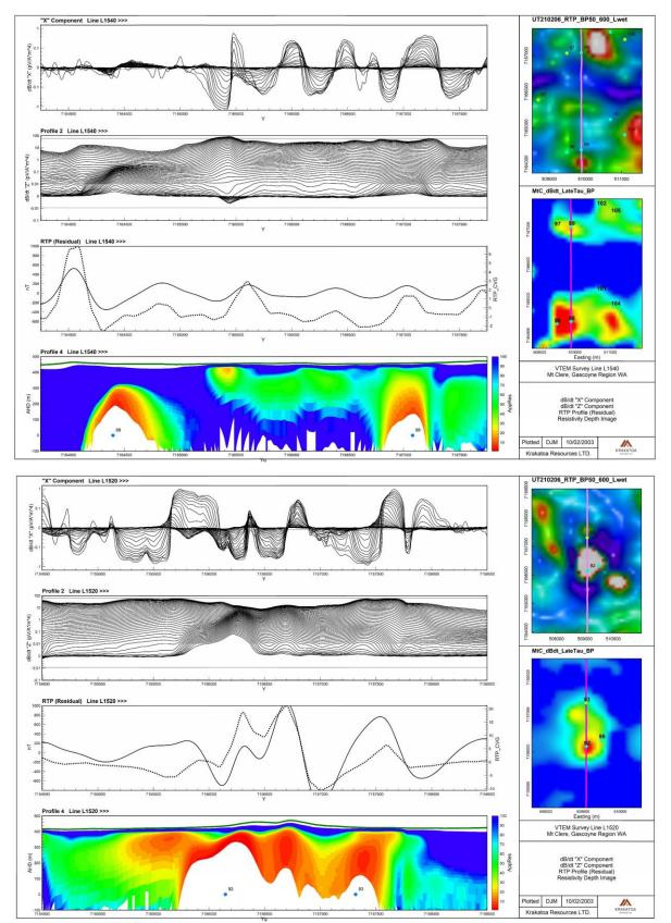
**Figure 3** Section plots through the Bullbadger cluster - Line 1540 (top) and Milly Milly cluster - Line 1520 (bottom). Each Plot displays "X' and "Z" component observed data time decay profiles, Total magnetic field and derivative profiles (Reduced To Pole) with Resistivity Depth transform images. The equivalent profile length is displayed in plans over the residual Reduced to pole magnetic image and late time Tau image.
