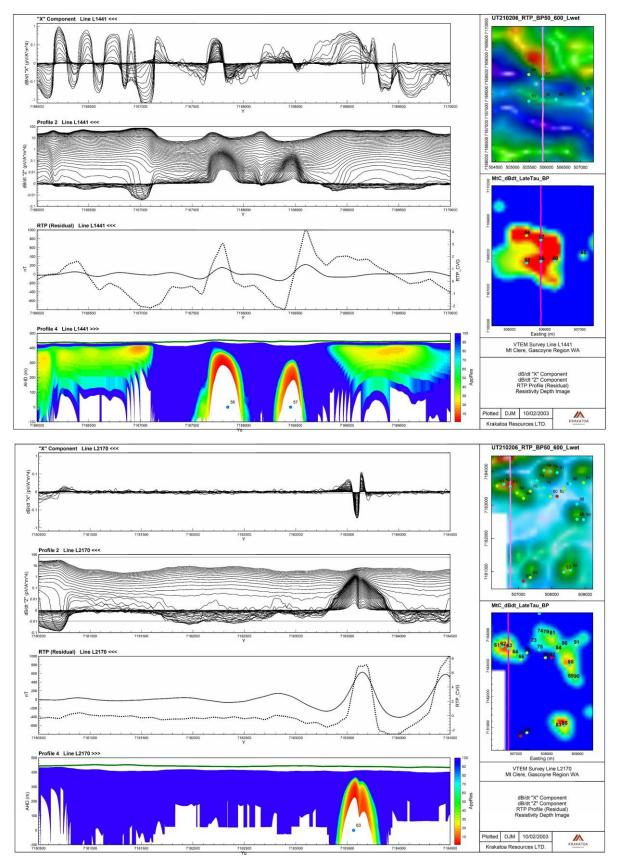
**Figure 2** Section plots through Calvin cluster - Line 1441 (top) and K-13 cluster - Line 2170 (bottom). Each Plot displays "X" and "Z" component observed data time decay profiles, Total magnetic field and derivative profiles (Reduced To Pole) with Resistivity Depth transform images. The equivalent profile length is displayed in plans over the residual Reduced to pole magnetic image and late time Tau image.
