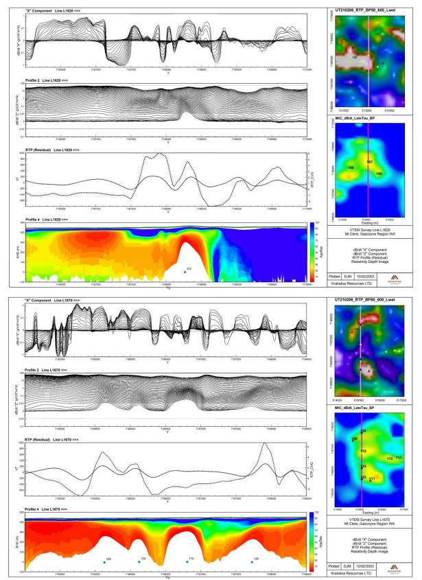
**Figure 4** Section plots through the North Bullbadger (NBB) cluster, showing Lines 1620 (top) and 1670 (bottom). Each Plot displays "X' and "Z" component observed data time decay profiles, Total magnetic field and derivative profiles (Reduced To Pole) with Resistivity Depth transform images. The equivalent profile length is displayed in plans over the residual Reduced to pole magnetic image and late time Tau image.
