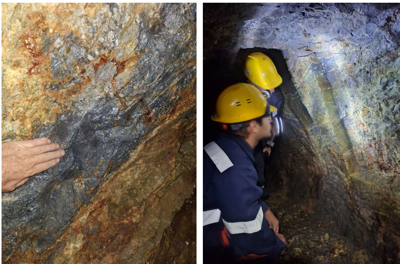
Photograph 1 and 2: (Left) Exposed antimony rich vein within adit 80 were 2014 channel sample #2010_V-6_A80_2014 which returned 22.6% Sb and 3.23g/t Au from the 70cm channel. (Right) Krakatoa geological team inspecting the adit and channel sample cuts.
