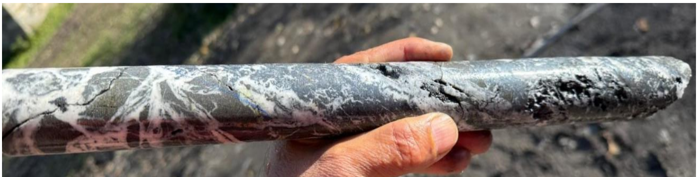
Figure 1 Core from drillhole UG25ZOP003 (~7.3m depth) showing the vein system with a zone of quartz - sulphide breccia. Antimony sulphides (Stibnite \text{Sb}_2\text{S}_3 ) in this interval constitute ~30% of the rock shown. Assays are pending for this interval and are expected December 2025 to January 2026.
