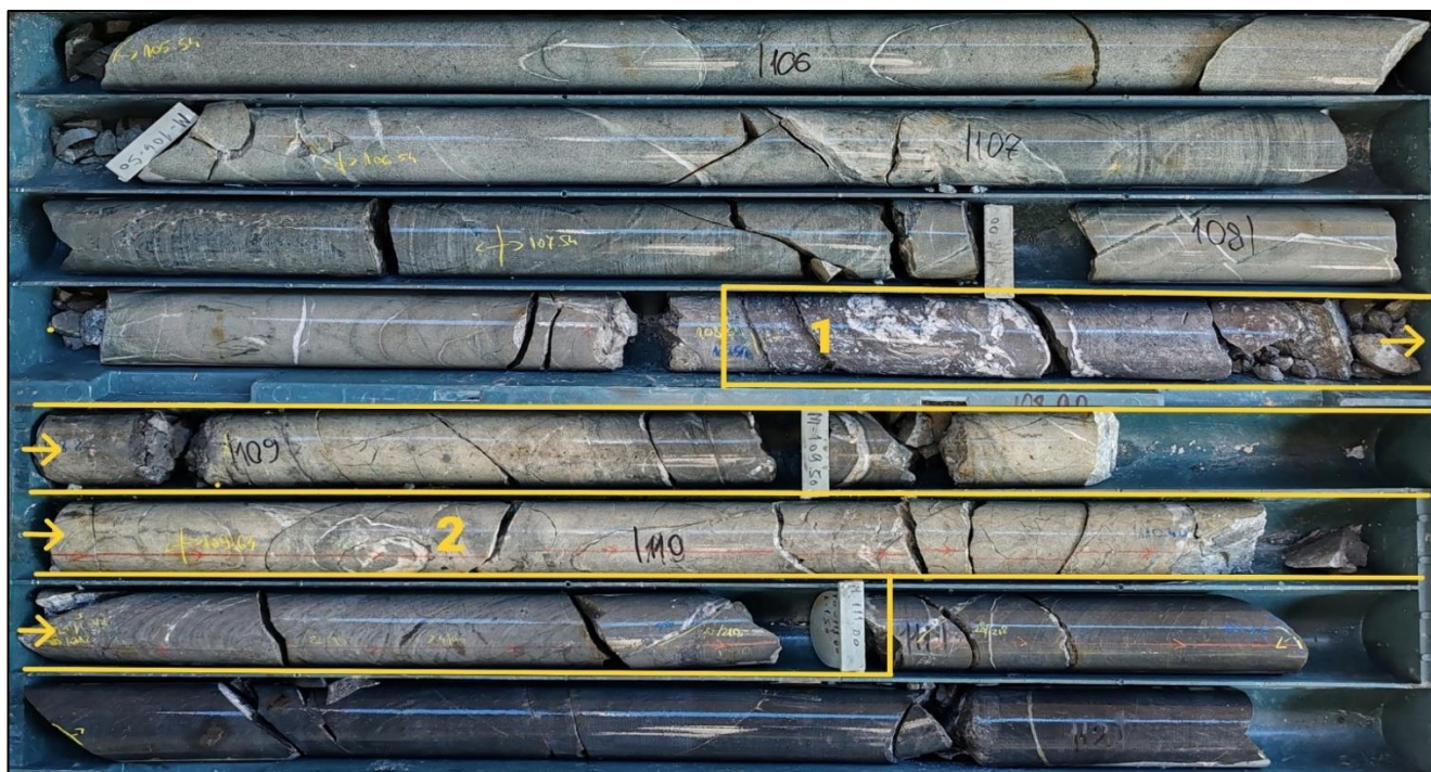
Figure 5 Photo of the mineralised antimony zones (yellow box) within drillhole DD25ZOP014 showing massive stibnite and quartz (~90% antimony) zone transitioning stringer veins of quartz – sulphide – stibnite within the parent rock (noted by 2). Drilling prior to the antimony zone is enriched in arsenopyrite sulphide alteration which may contain gold. Drilling stopped in antimony rich mineralisation. Assays are pending for this hole and are expected in December 2025 to January 2026. Note: Visual estimates of mineral abundance should never be considered a proxy or substitute for laboratory analyses where concentrations or grades are the factor of principal economic interest. Visual estimates also potentially provide no information regarding impurities or deleterious physical properties relevant to valuations.
