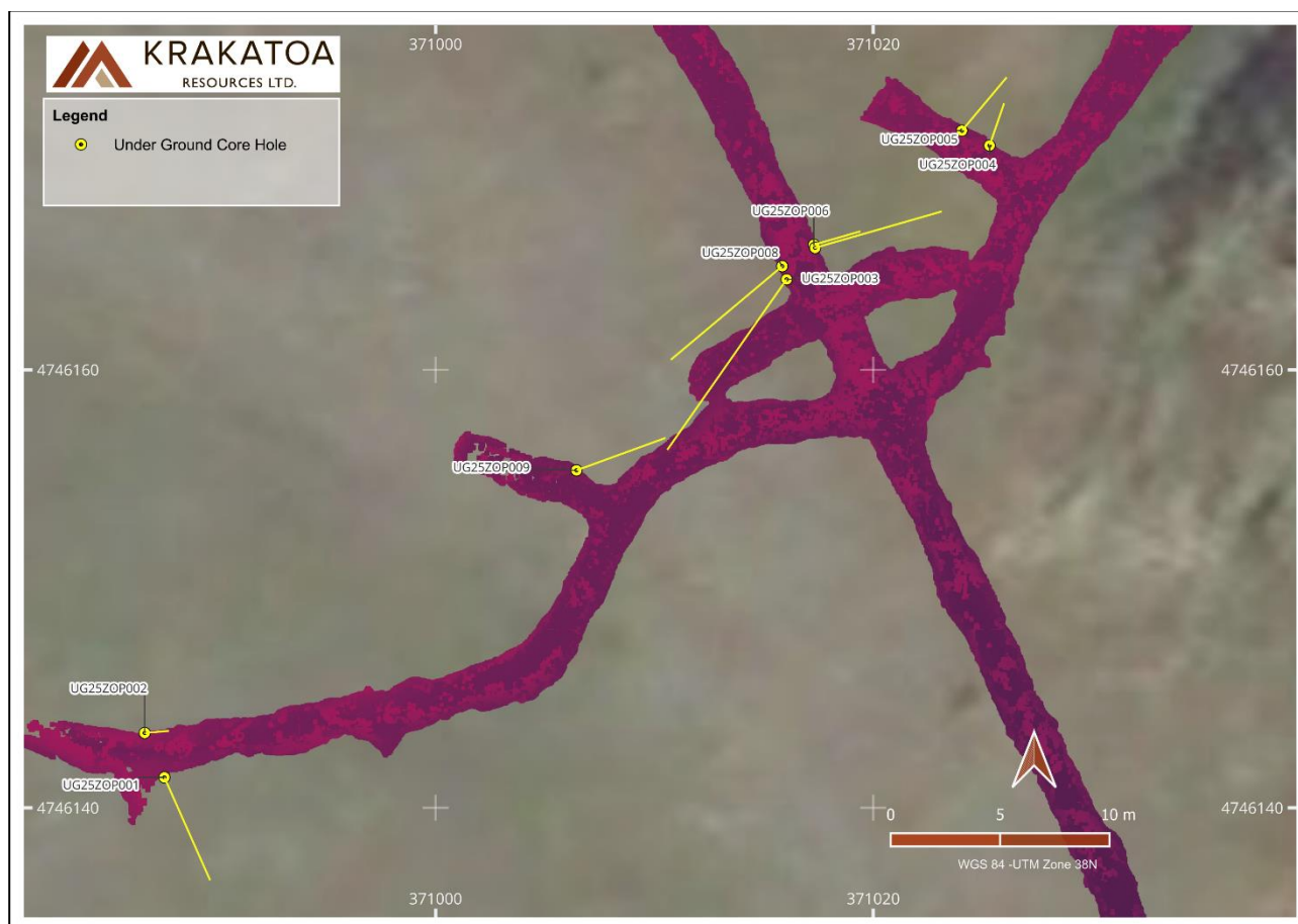
Figure 3 Plan view showing the locations of the underground core sampling drill holes in relation to the adit LiDAR surface profile.
