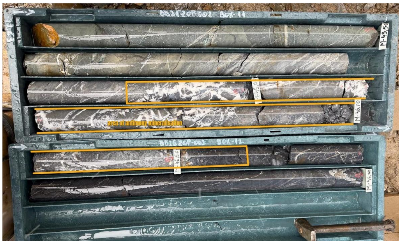
Figure 3 Photo of the mineralised antimony zones (yellow box) within drillhole DD26ZOP-002 showing breccia of quartz with stibnite filling veins and vugs (~25% Stb) at start, transitioning to a massive stibnite (0.6m of ~50% Stb). Drilling prior to the antimony zone is enriched in arsenopyrite sulphide alteration which may contain gold. Assays are pending for this hole.
