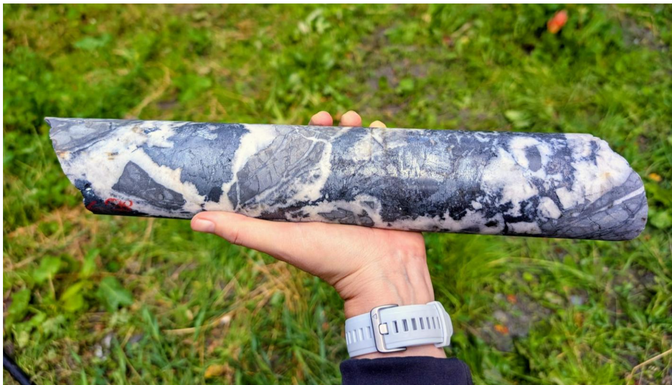
Figure 1 Photograph of 44cm long drill core from hole DD26ZOP-002 (interval 44.66 – 45.00m) showing stibnite (antimony mineral) (estimated ~25%), slate and quartz breccia with disseminated sulphides. Assays are pending for this interval. Visual estimates of mineral abundance should never be considered a proxy or substitute for laboratory analyses where concentrations or grades are the factor of principal economic interest. Visual estimates also potentially provide no information regarding impurities or deleterious physical properties relevant to valuations.
