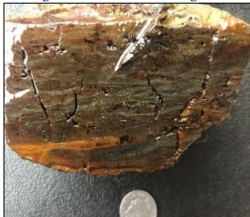
Photo 9: Trough Gully Mine foliated sulphide veining – evidence of boudinage structures
