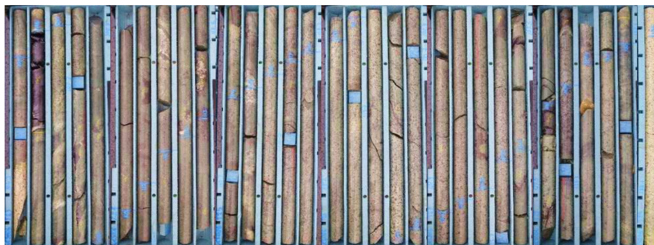
Photo 3: Drill hole WCS006: mineralised intercept 27.50m @ 468 g/t AgEq (or 9.60 % ZnEq) from 104.6m
