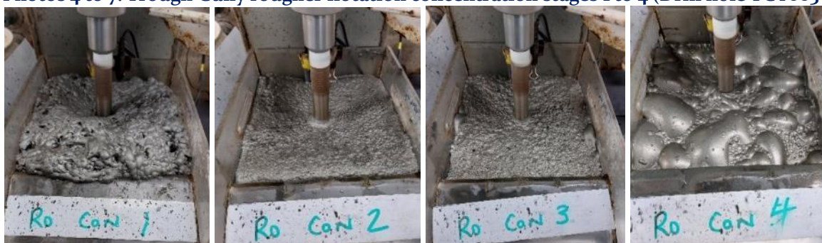
Photos 4 to 7: Trough Gully rougher flotation concentration stages 1 to 4 (Drill hole TGY003)
