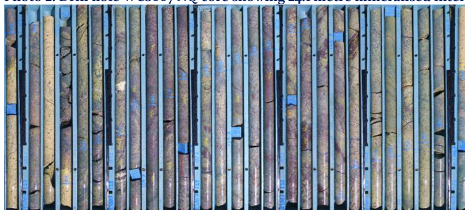
Photo 2. Drill hole WCS007 NQ core showing 24.1 metre mineralised intercept
