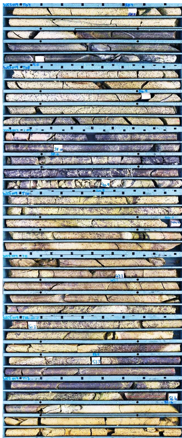
Photo 3: NQ core showing 26.5m mineralised intercept from drill hole WCS019 at Tangoa West prospect
