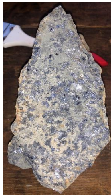
Photo 4: Webbs Consol Main Shaft specimen showing coarse galena mineralisation
