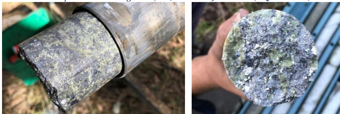
Photos 1 &amp; 2: Very coarse blebs of galena (PbS) in WCS019 drill core (NQ2 core size)
