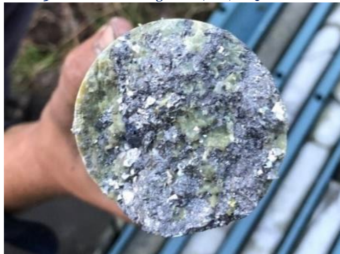
Photo 3: Coarse blebs of galena (PbS) NQ 2 size drill core at Webbs Consol
