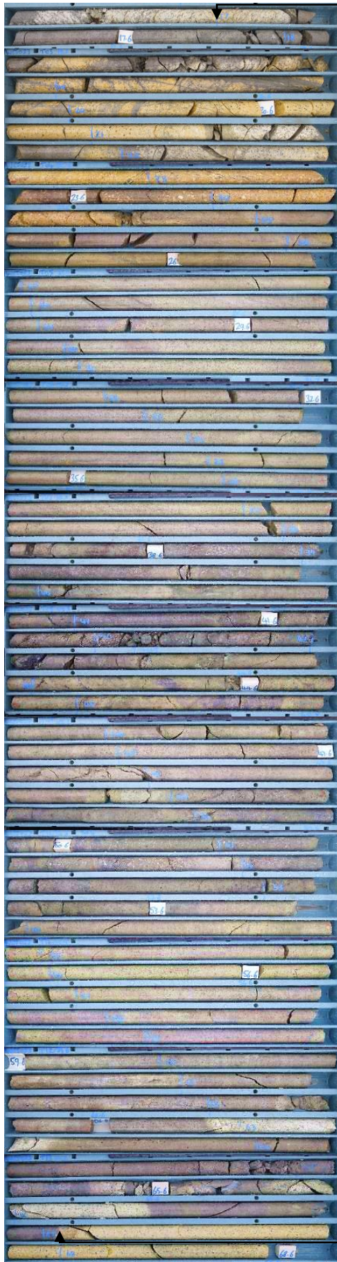
Photo 1: NQ core showing 50.0m sulphide intercept from drill hole WCS023 at Castlereagh prospect
