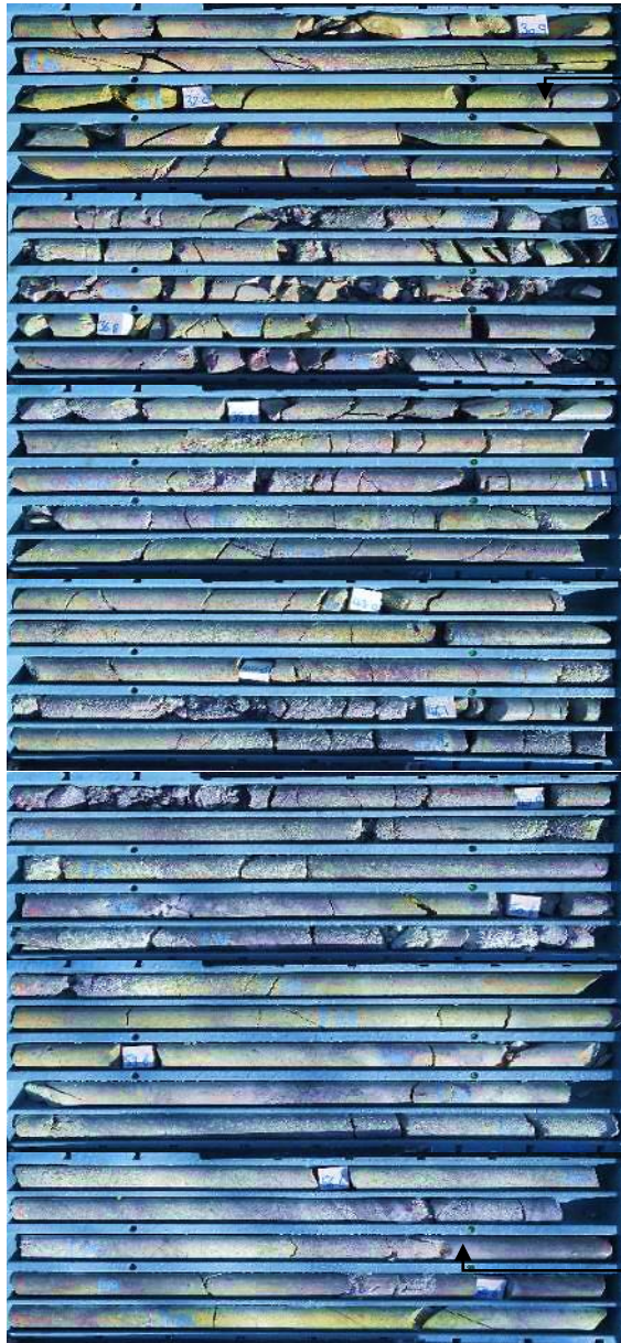
Photo 2: NQ core showing 26.1 sulphide intercept from drill hole WCS026 at Lucky Lucy North prospect
