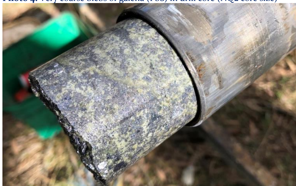
Photo 4: Very coarse blebs of galena (PbS) in drill core (NQ 2 core size)
