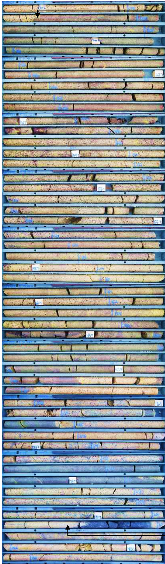
Photo 3: NQ core showing 42.0m sulphide intercept from drill hole WCS028 at Main Shaft prospect
