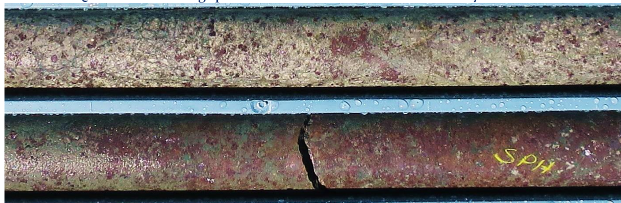
Photo 2: NQ drill core showing sphalerite rich mineralisation in WCS0007 at Webbs Consol
