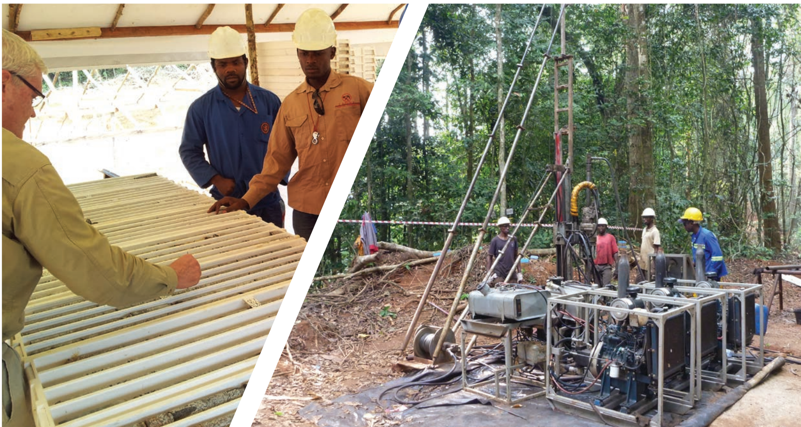
Man Portable Diamond Drilling Rig – Melombo East.
