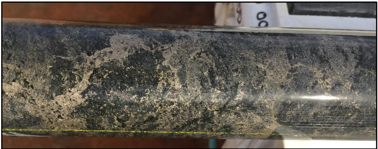
Photo 1: RKDD001-566.8m: Pyrrhotite in mafic granulite (NQ2 core)
