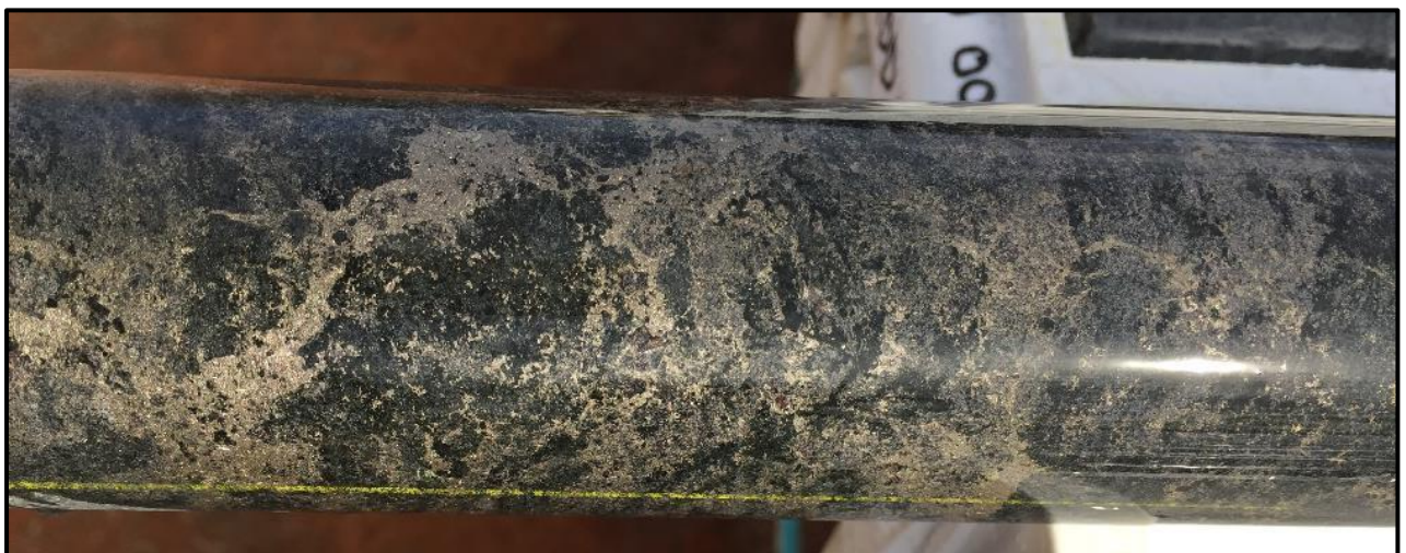
Photo 1: RKDD001-566.8m: Pyrrhotite in mafic granulite (NQ2 core)
