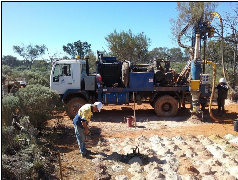
Aircore Drilling at Rockford Project
