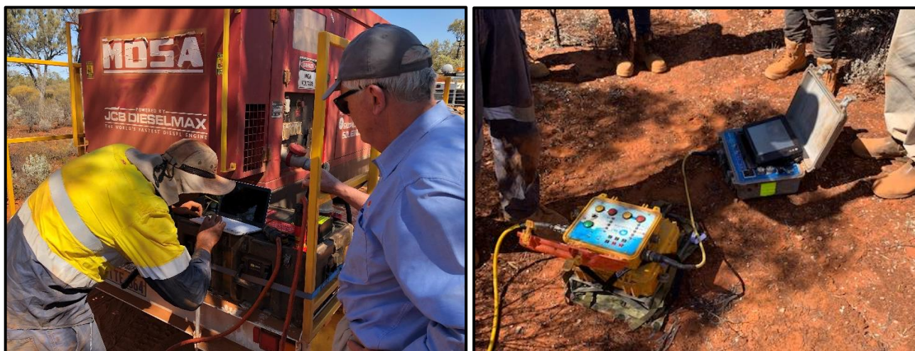
Area D: Low Frequency MLTEM Survey (Left) Generator/transmitter set up, (Right) Data Recording Instrumentation
