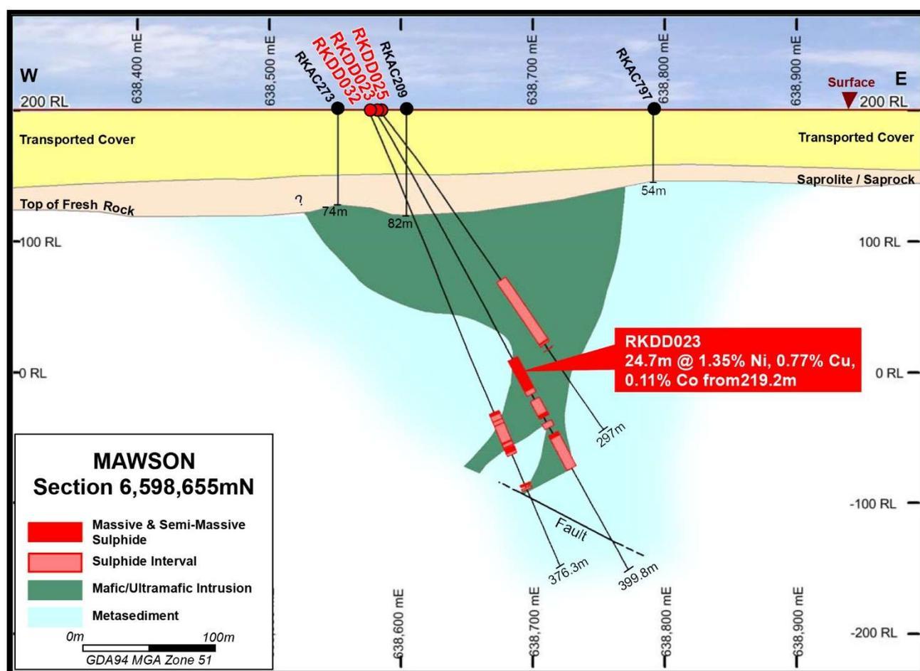
Figure 3: Drill Section 6,598,655N Showing Diamond Drillholes RKDD023, RKDD025, & RKDD032
