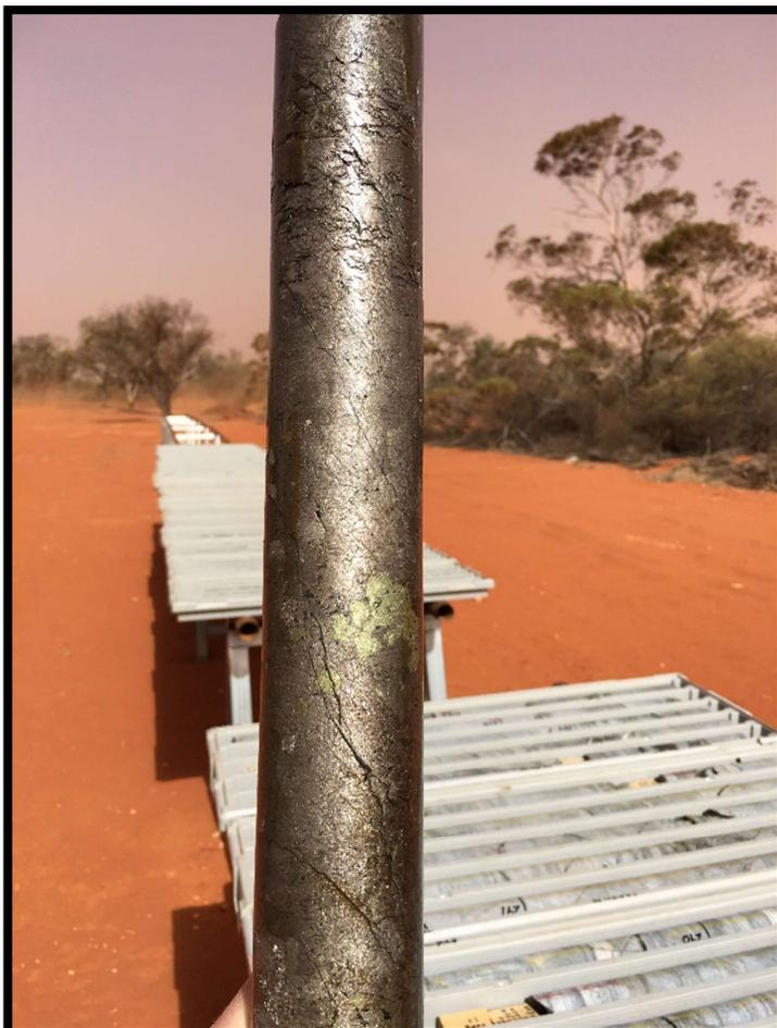
*Massive Ni-Cu Sulphide from RKDD032 from 274m, NQ2*
