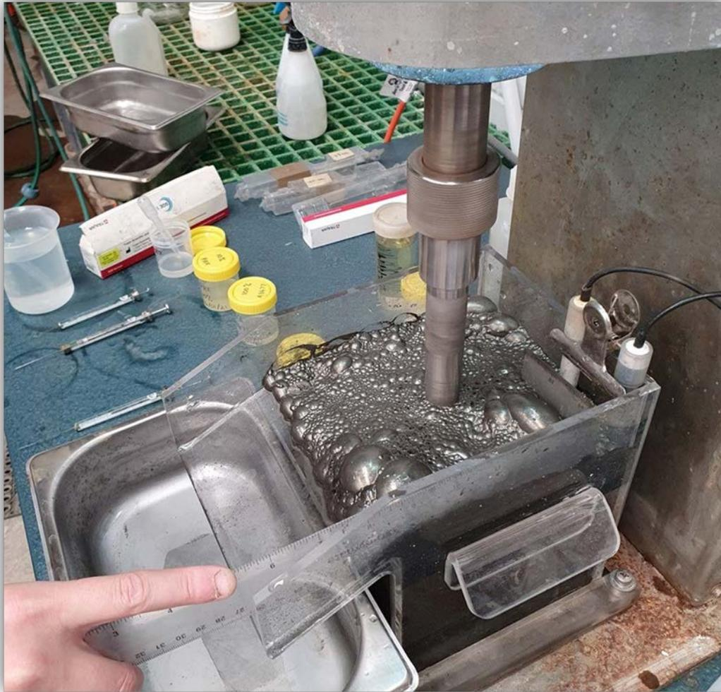
**Flotation Test Work of RKDD034
