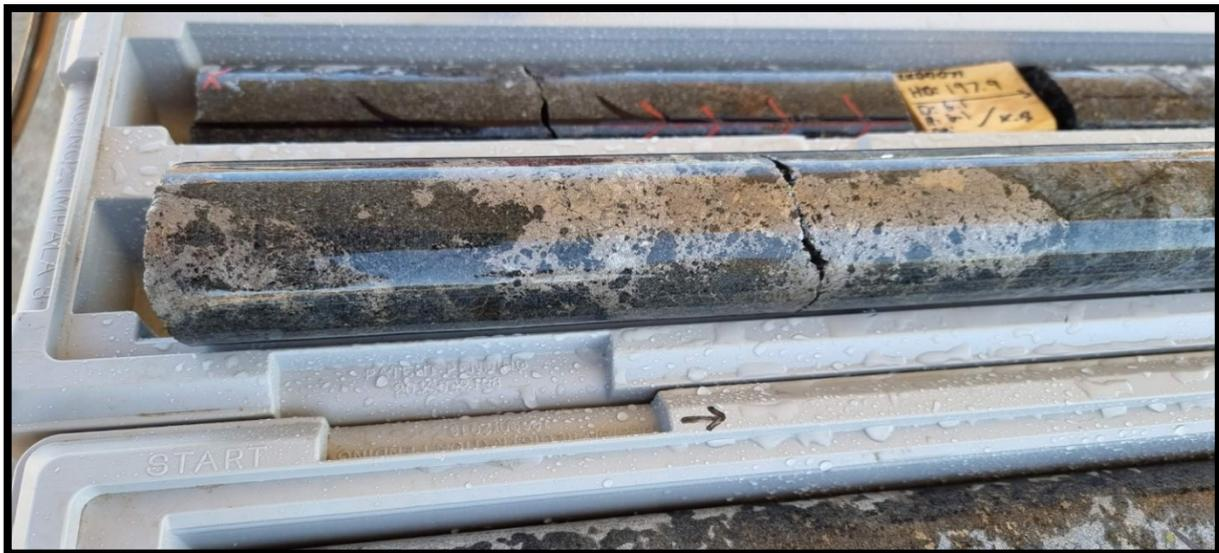
**Photo 4: Ni-Cu sulphide mineralisation from RKDD71 from 201m**
