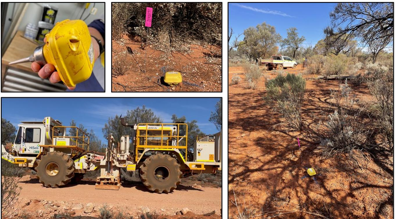
**Photos: HiSeis Seismic Survey Vibe Truck and Geophone Receivers at Mawson**
