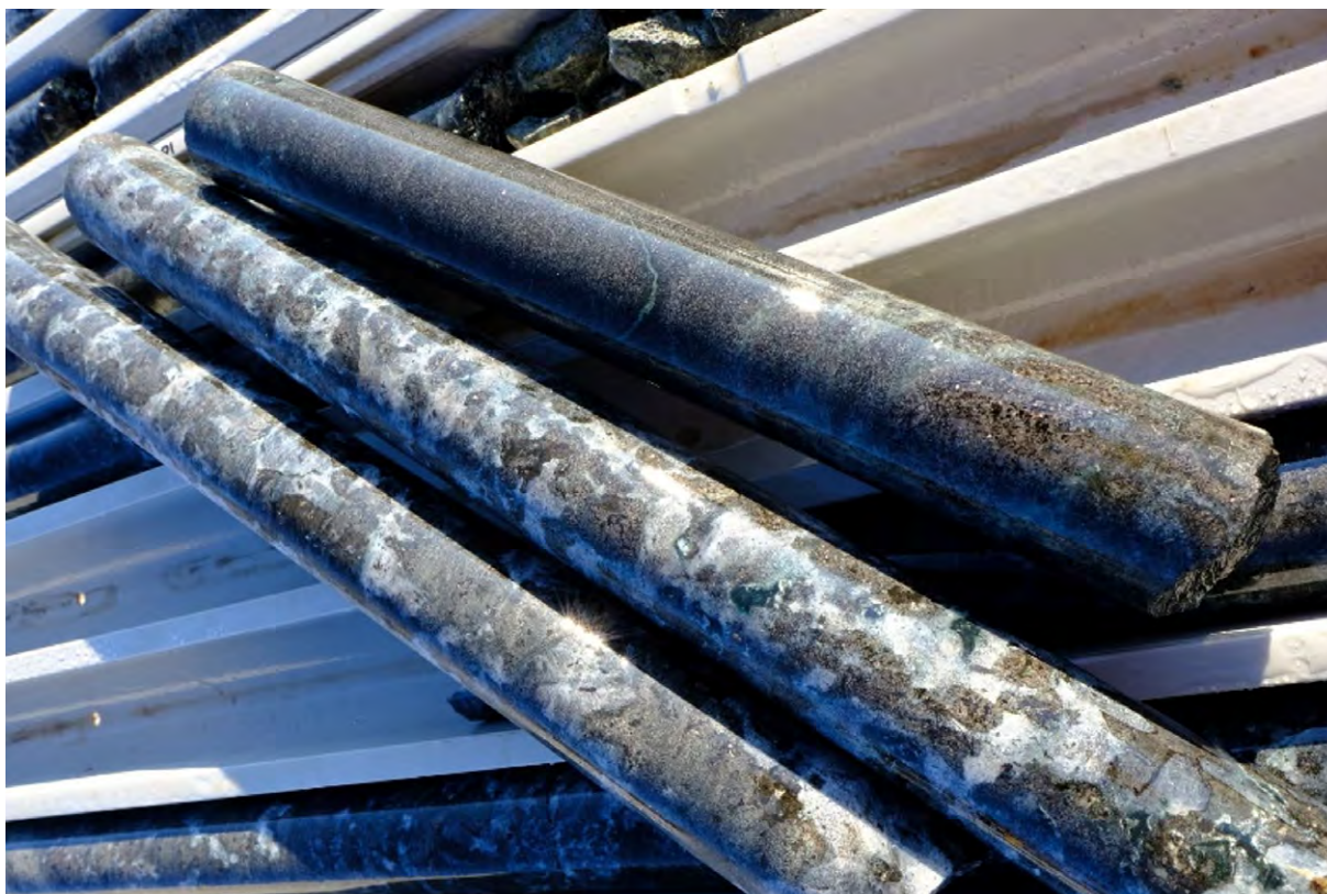
PHOTO 3: TEXTURAL AND LITHOLOGICAL VARIATIONS OF INTRUSIVES INTERSECTED WITH VARIABLE MINOR SULPHIDE MINERALISATION FROM MGDD01 AT THE MAGNUS PROSPECT.
