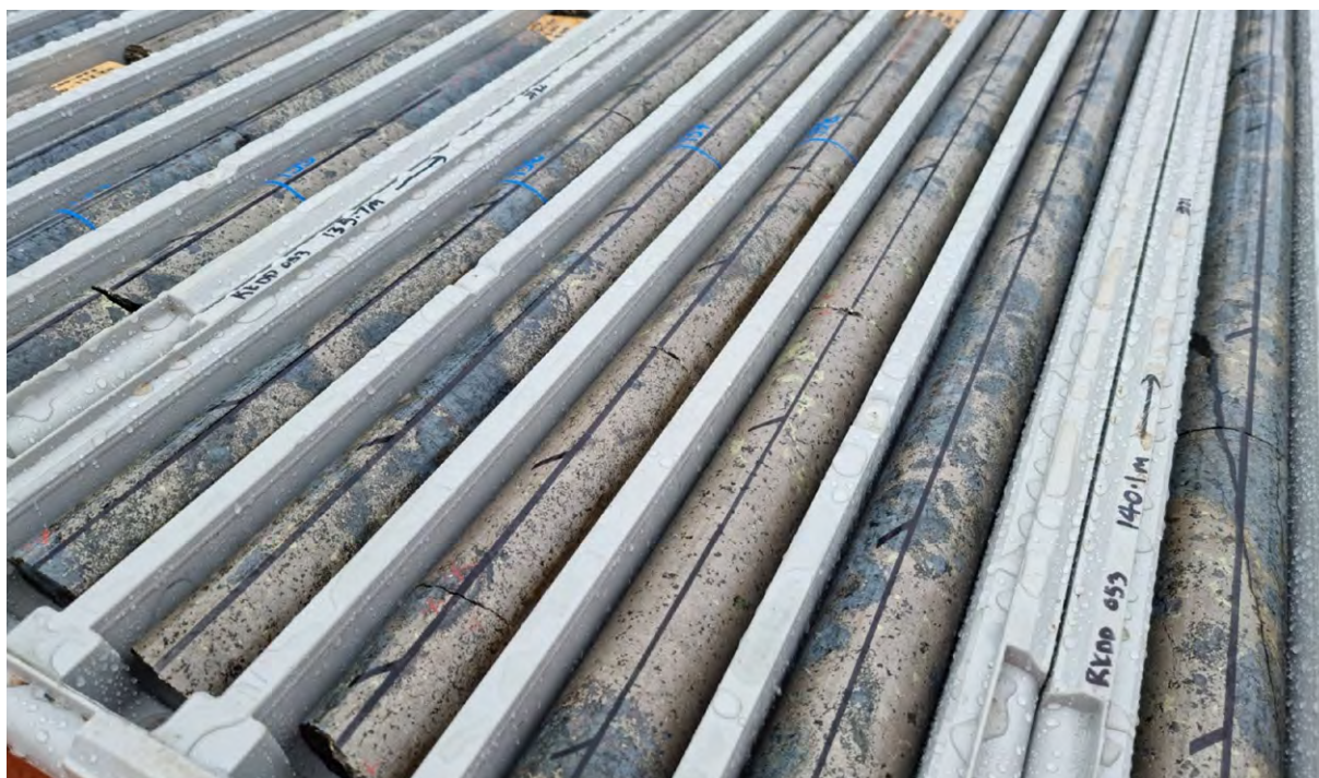
PHOTO 1: MASSIVE AND SEMI-MASSIVE NI-CU SULPHIDE FROM RKDD053 FROM 135M
