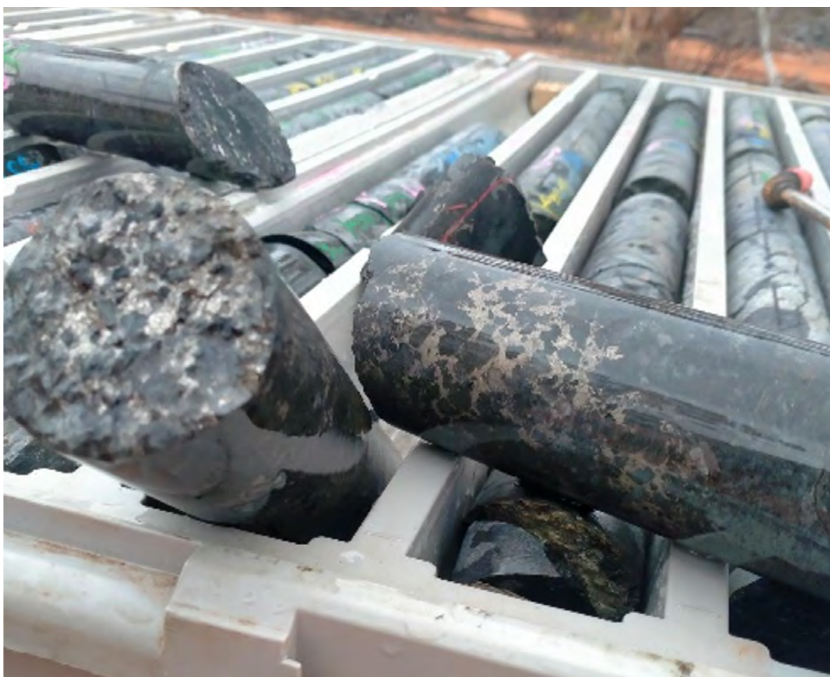
PHOTO 4: STRINGER AND BLEBBY PYRRHOTITE AND CHALCOPYRITE SULPHIDES WITH DISSEMINATED GRAPHITE WITHIN OLIVINE LEUCONORITE FROM HYDD002 FROM 415.85M.
