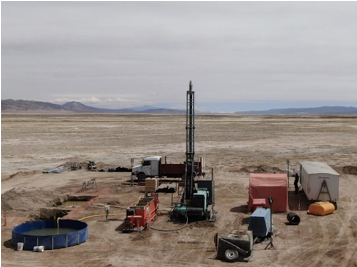
Figure 2: Second Diamond Drill Rig at SOZDD003, Chico I Concession on Olaroz Salar
