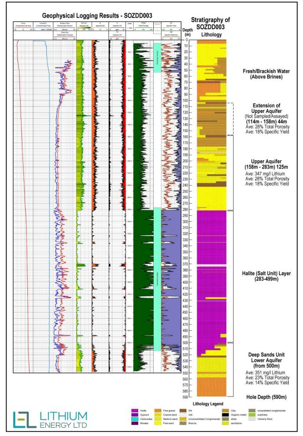
Figure 3: Geophysical Hole Logging Results and Drillhole Stratigraphy for SOZDD003
