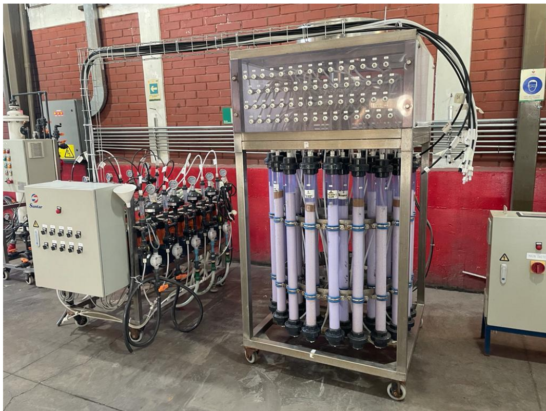
Figure 1: Lanshen Laboratory Scale Continuous Operation Carousel with Lithium Adsorbent
