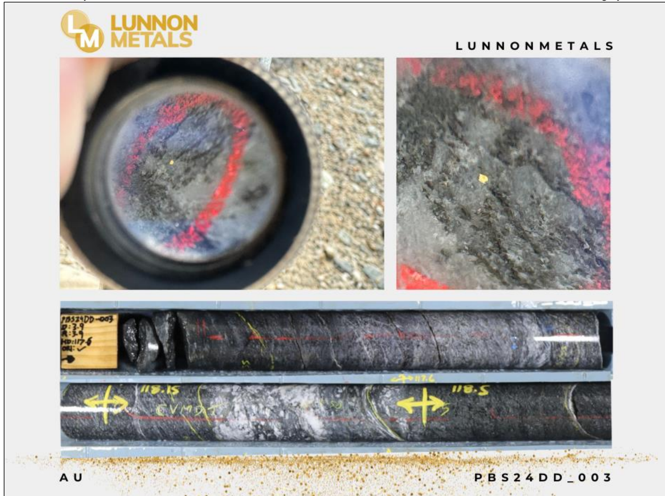
Figure 4: Photograph of DD hole PBS24DD_003 depicting fine free gold identified during logging at 117.9m.
