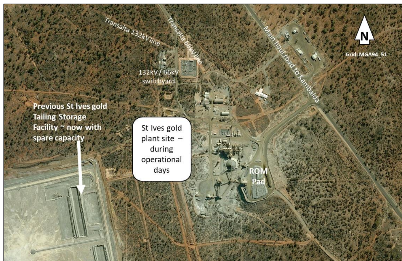
Figure 2: Zoomed-in plan view of the previous St Ives gold plant site during its operational life, associated tailing storage facility and supporting infrastructure.
