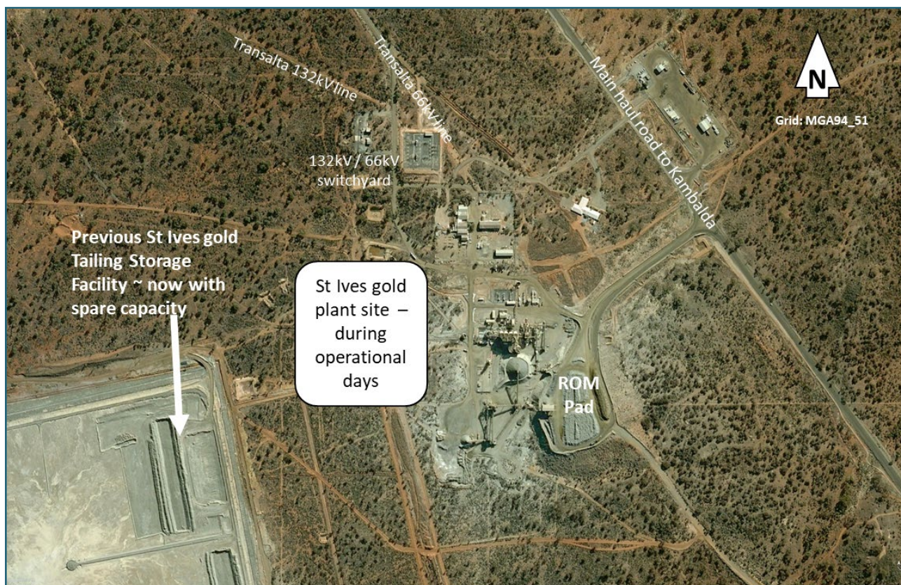
Figure 19: Zoomed-in plan view of the previous St Ives gold plant site during its operational life, associated tailing storage facility and supporting infrastructure.
