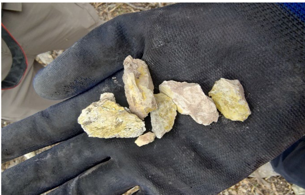
Figure 1. Field photo of outcrop sample MQ12 from the Eridani target containing carnotite mineralisation.
