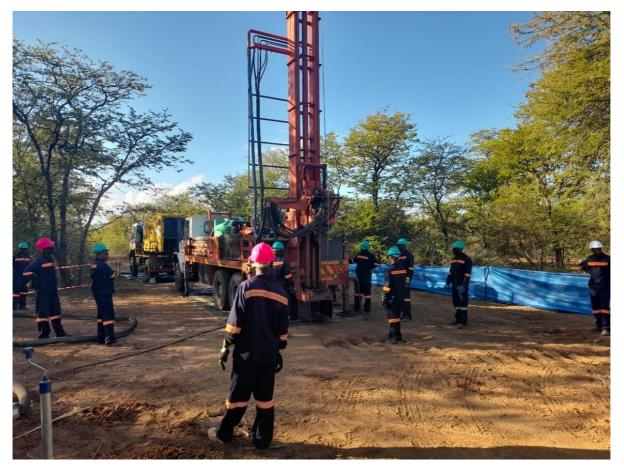
Figure 2: RC rig on site at Letlhakane
