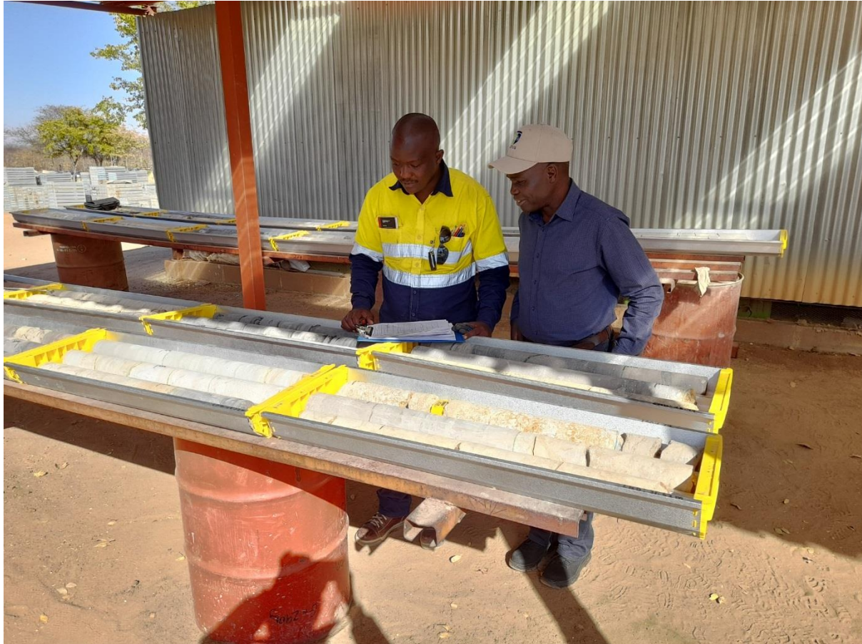
Figure 6: Lotus Resources geologists examining PQ sized diamond drill core from Serule West at the company's core storage yard.
