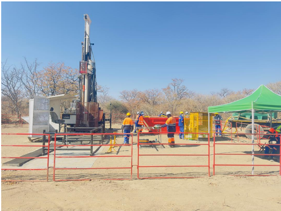
Figure 5: Boart Longyear LF90 diamond coring rig set up at Serule West.
