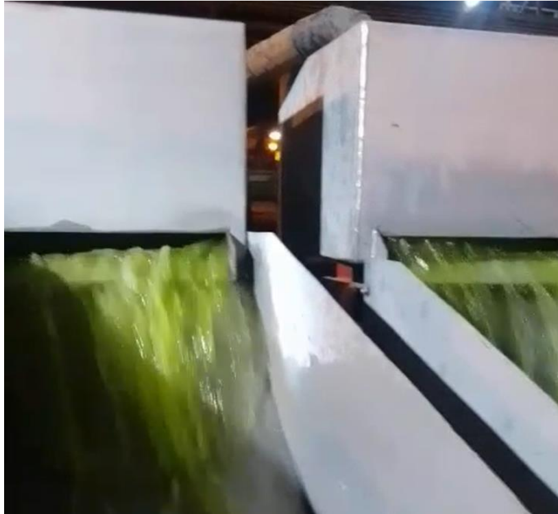
Figure 4: Clean uranium eluate into storage before delivery to precipitation
