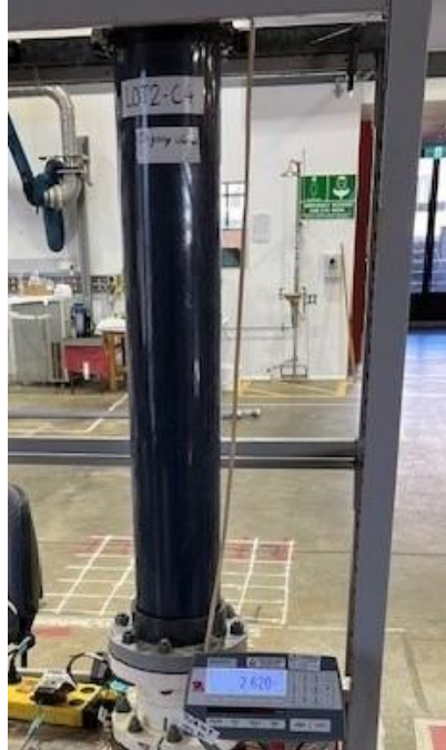
Figure 1: Column heap leach test set up
