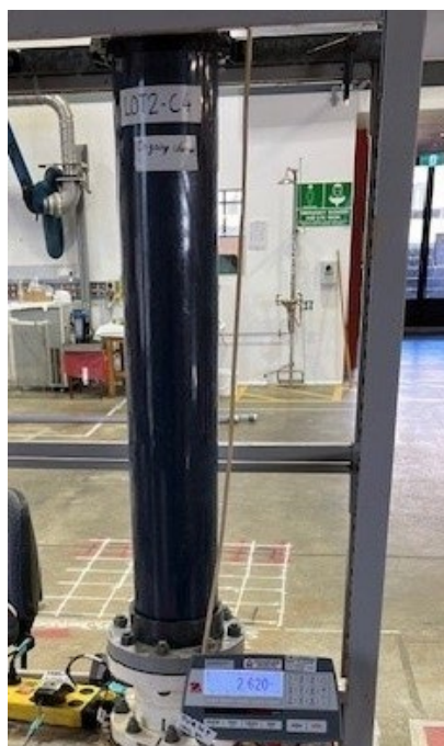
Figure 13: Column heap leach test set up
