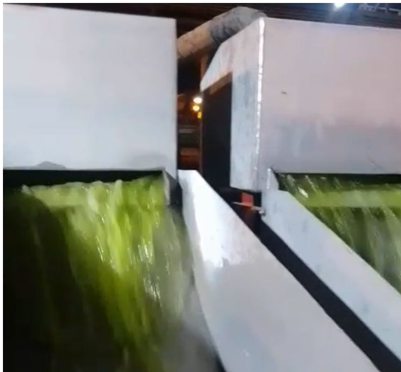
Figure 6: Clean uranium eluate into storage before delivery to precipitation
