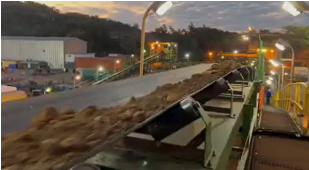
Figure 3: Mill feed conveyor in operation
