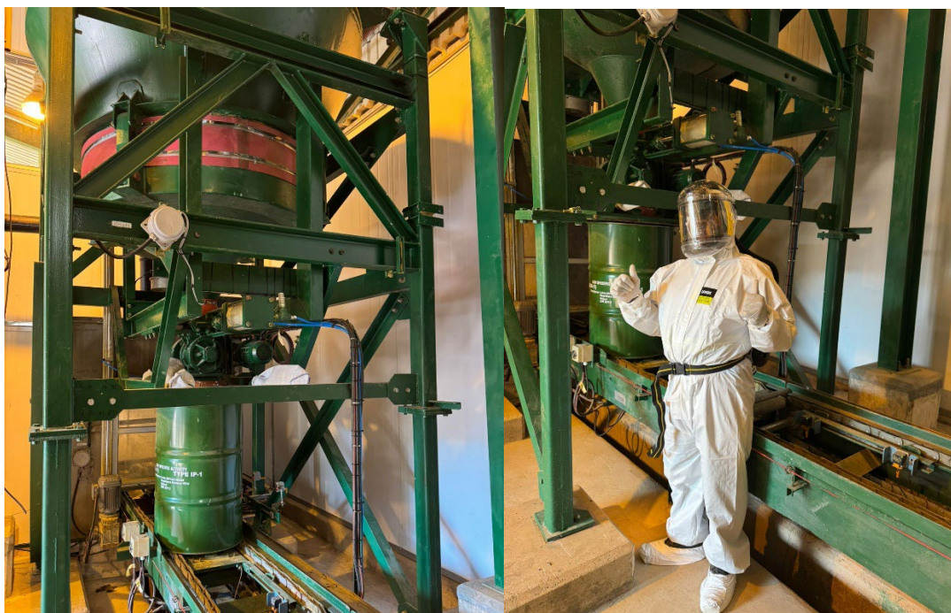
Figure 2: Yellowcake being drummed at Kayelekera's packaging and drying plant
