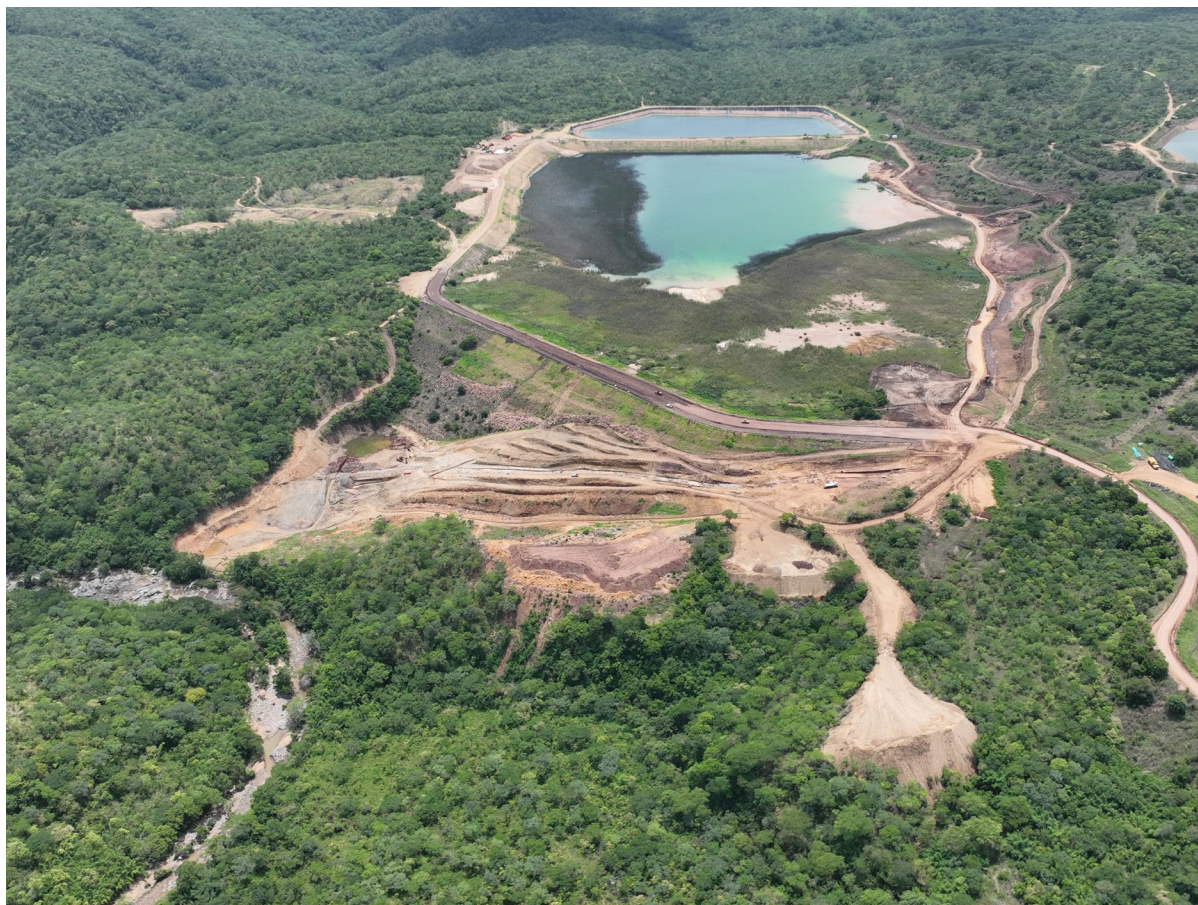
Figure 5: TSF lift works in progress
