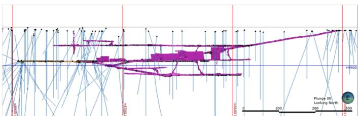
Figure 9 - View to the north presenting the depleted development and production wireframes (magenta).
