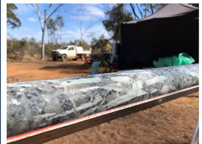
Buldania drill core showing coarse spodumene crystals
