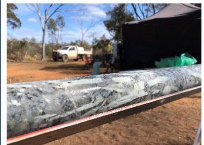
Buldania drill core showing coarse spodumene crystals
