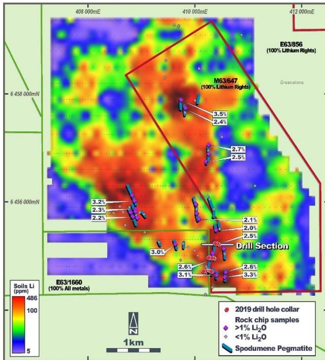
**FIGURE 8: BULDANIA PROJECT/NW PEGMATITE AREA – LITHIUM IN SOIL IMAGE SHOWING PEGMATITES, ROCK CHIP SAMPLING AND MAIDEN DRILL HOLES.**
