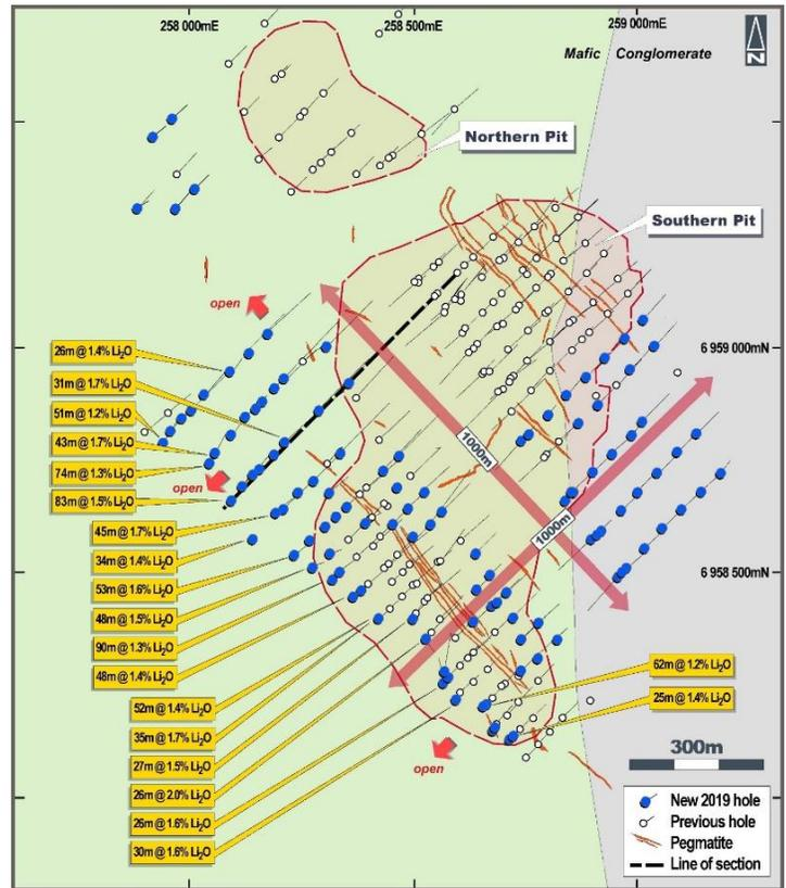
FIGURE 3: KATHLEEN VALLEY PROJECT – DRILL HOLE PLAN SHOWING BETTER LITHIUM INTERSECTIONS FROM 2019 DRILLING.
