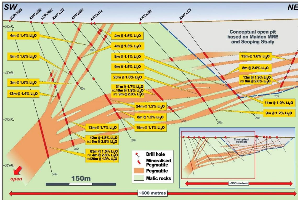
FIGURE 4: KATHLEEN VALLEY PROJECT – DRILL SECTION SHOWING MINERALISED PEGMATITES MERGING AT DEPTH (SEE FIGURE 3 FOR LOCATION).
