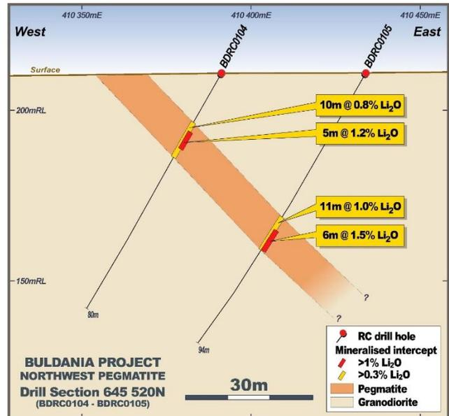
**FIGURE 9: BULDANIA PROJECT/NW PEGMATITE AREA – DRILL SECTION (SEE FIGURE 8 FOR LOCATION).**
