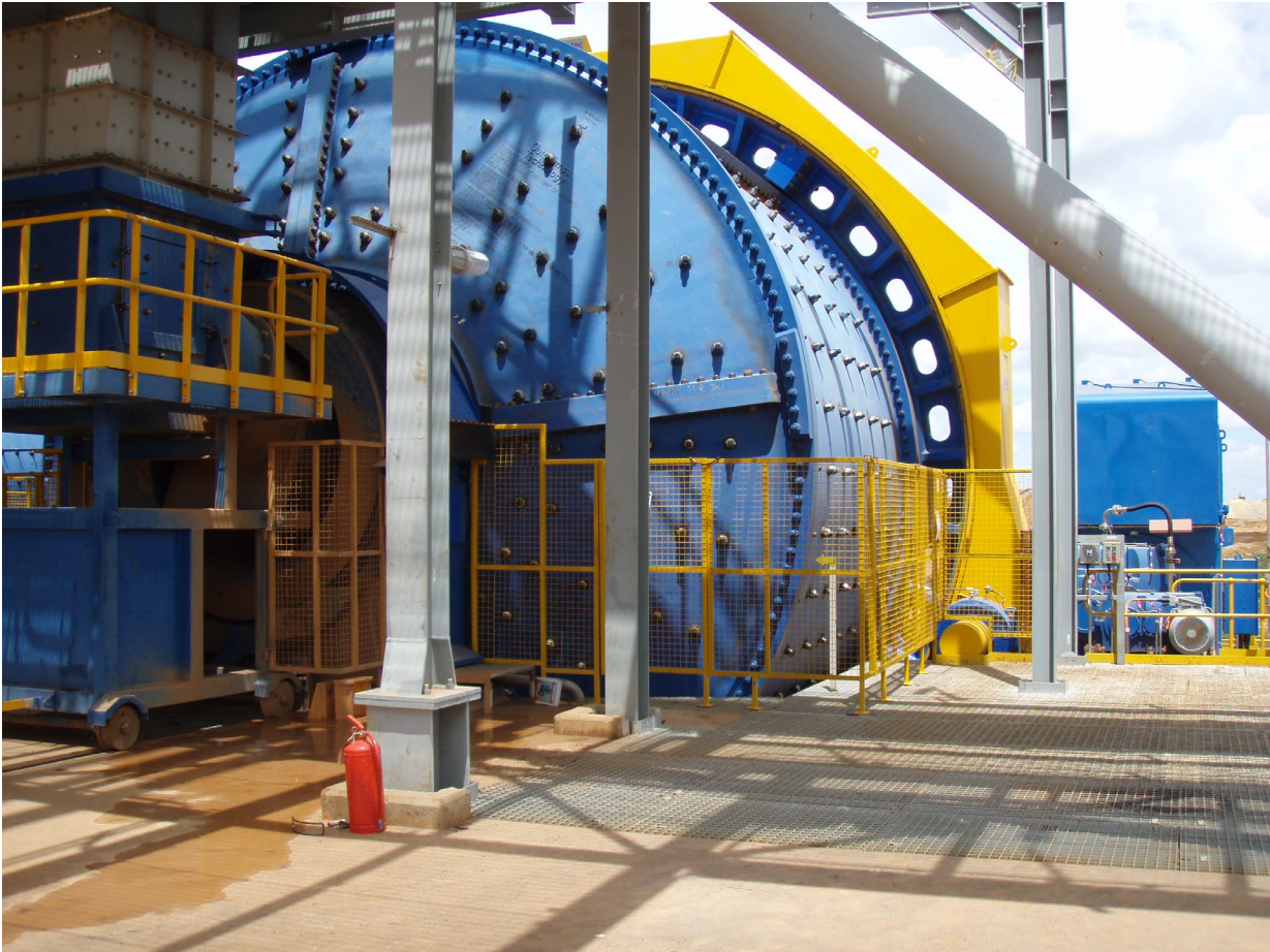
Figure 1: Example of installed Metso-Outotec Premier™ SAG Mill similar to the SAG Mill ordered.
