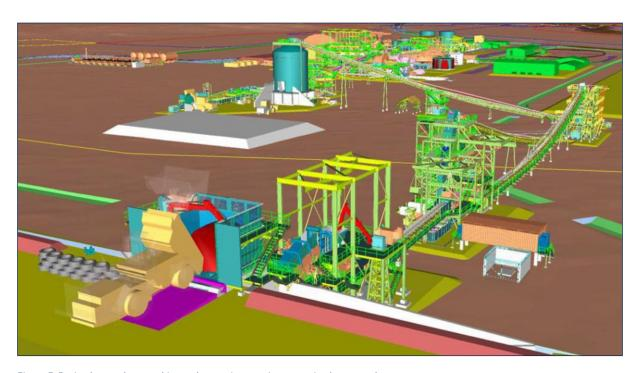
Figure 5: Revised secondary crushing and screening area incorporating lower steel heights and sacrificial conveyor on primary crushing area
