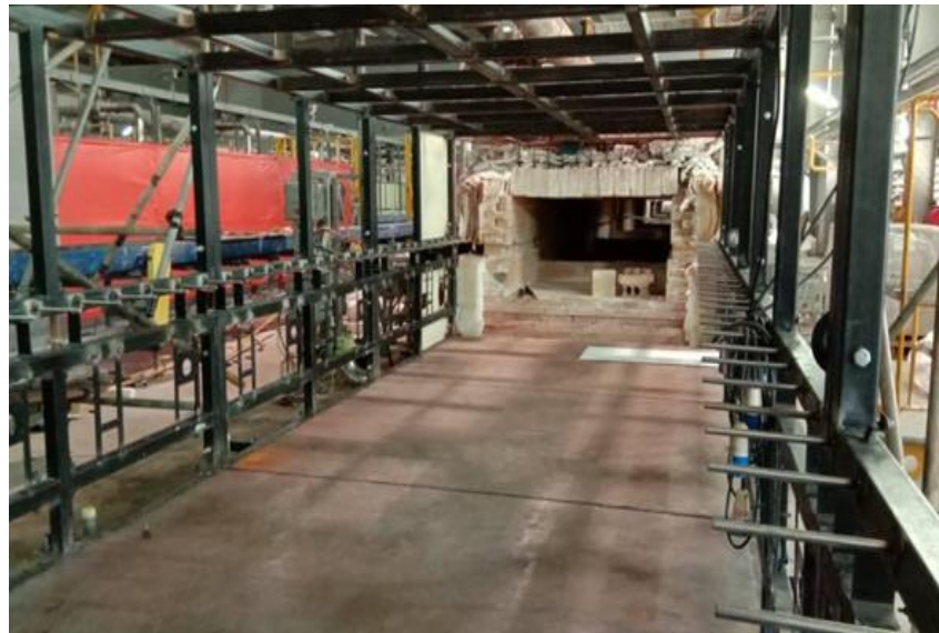
Tunnel Furnace 20A extension to increase calcination capacity
