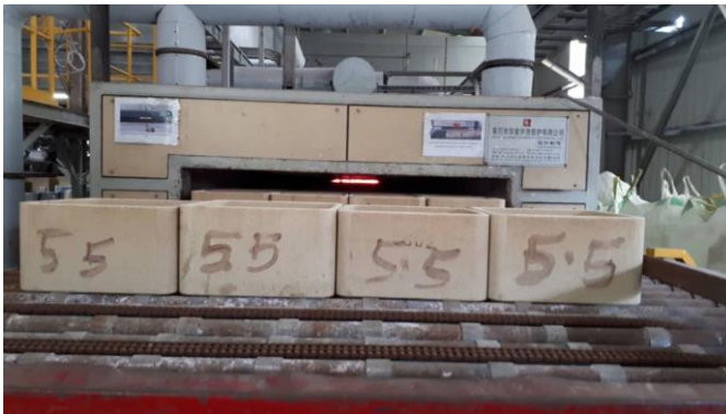
Trialling larger crucibles in Malaysian Tunnel Furnaces to improve capacity
