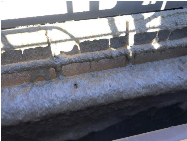
Cleaner 1 at Mt Weld, during reagent trial Froth is more fluid than normal
