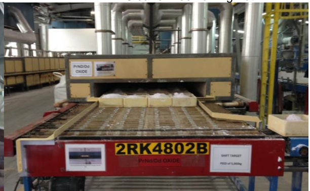
Trialling larger crucibles in Malaysian Tunnel Furnaces to improve capacity
