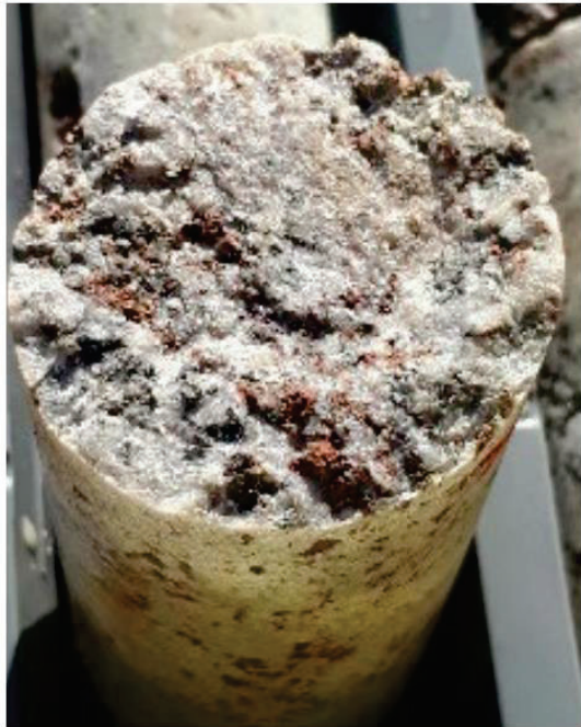
Brick red coloured coarse grained disseminated REE minerals at 748m depth-ankerite carbonatite host rock. The sample is part of a 4m drillhole composite from 747m to 751m has assayed 2.44% REO.
