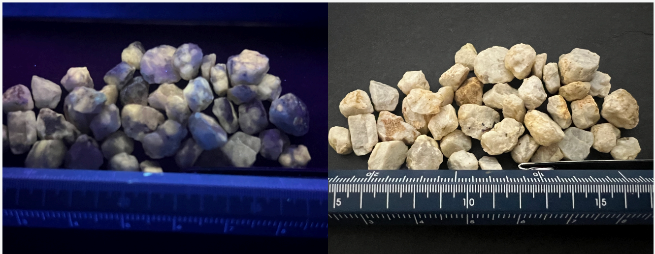
Figure 6. Pegmatite chips obtained from drill spoil at an historical Bullion Minerals RAB drill collar LJR034. Photograph taken under a long wave ultraviolet (UV) light source (left), and natural light (right). Scale bar is in centimeters.
