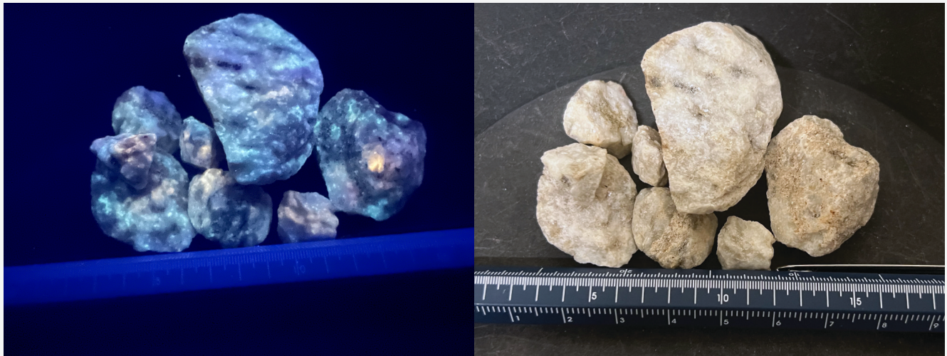
Figure 5. Pegmatite chips obtained from drill spoil at an historical Bullion Minerals RAB drill collar LJR010. Photograph taken under a long wave ultraviolet (UV) light source (left), and natural light (right). Scale bar is in centimeters.
