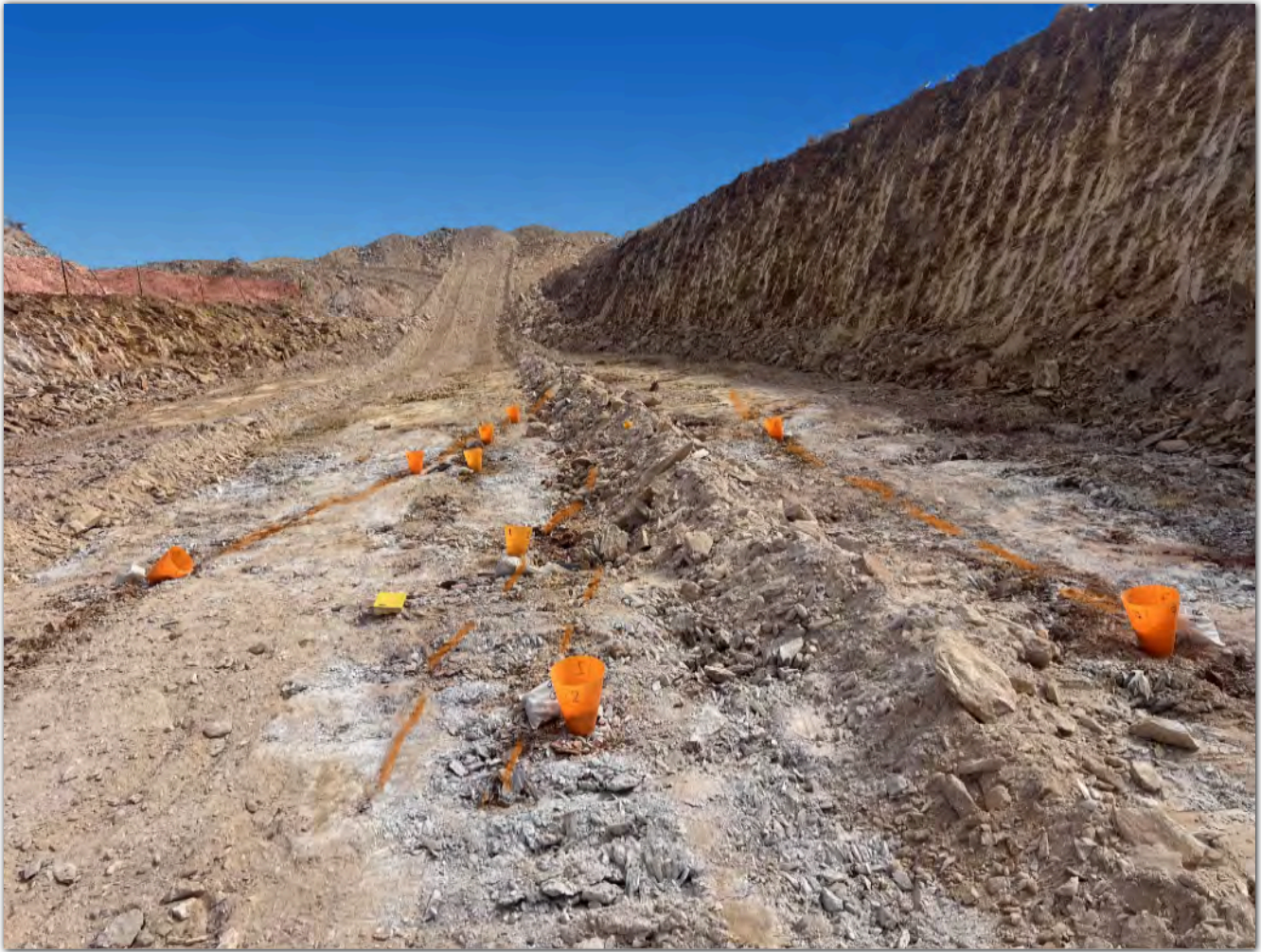
Picture 2: The orientation of mineralised quartz veins are indicated by orange lines drawn over the bulk sampling pit floor.
